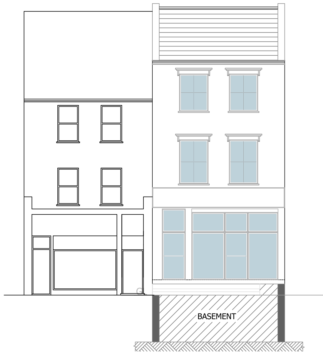
EXISTING FRONT ELEVATION
