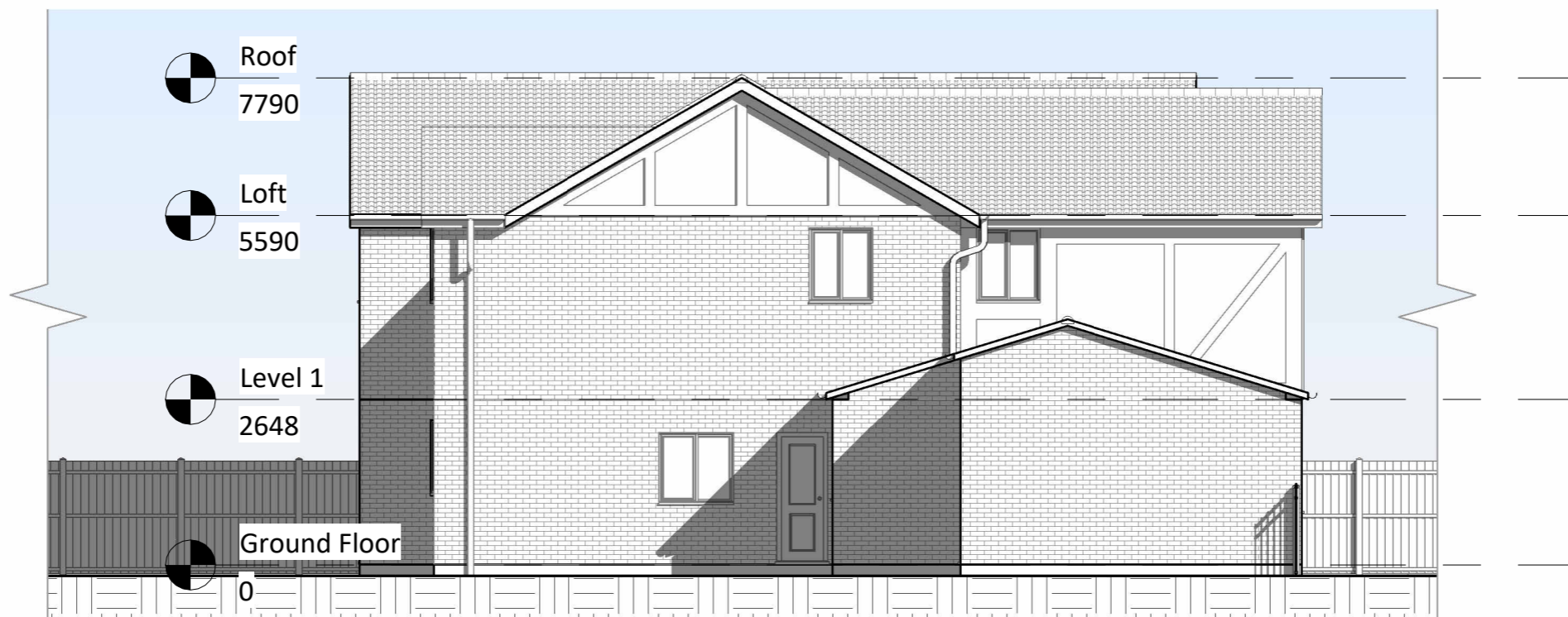
2 Proposed Left Elevation 1 : 100
