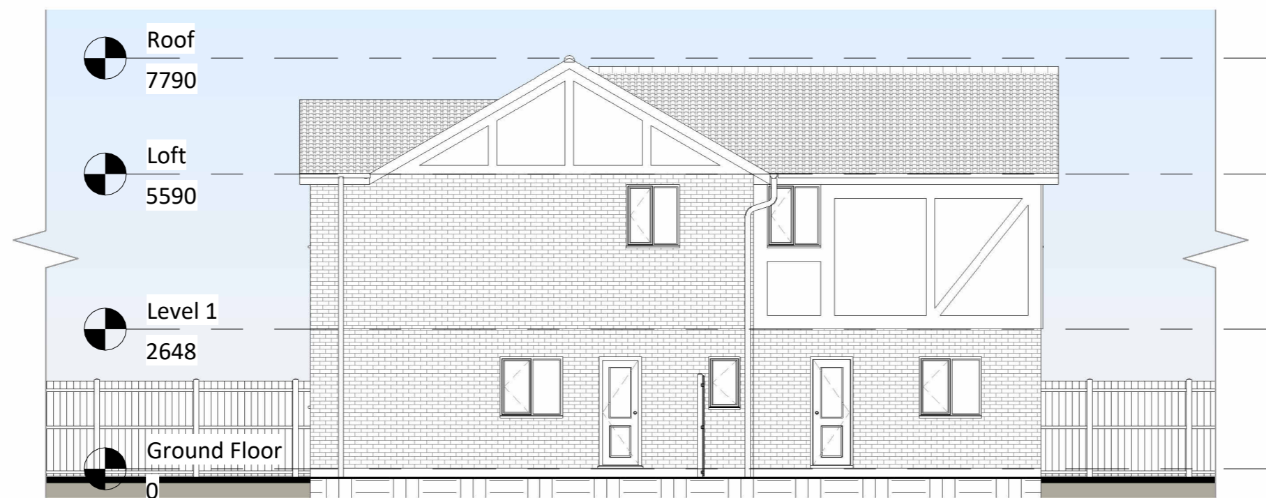
2 Existing Left Elevation 1 : 100
