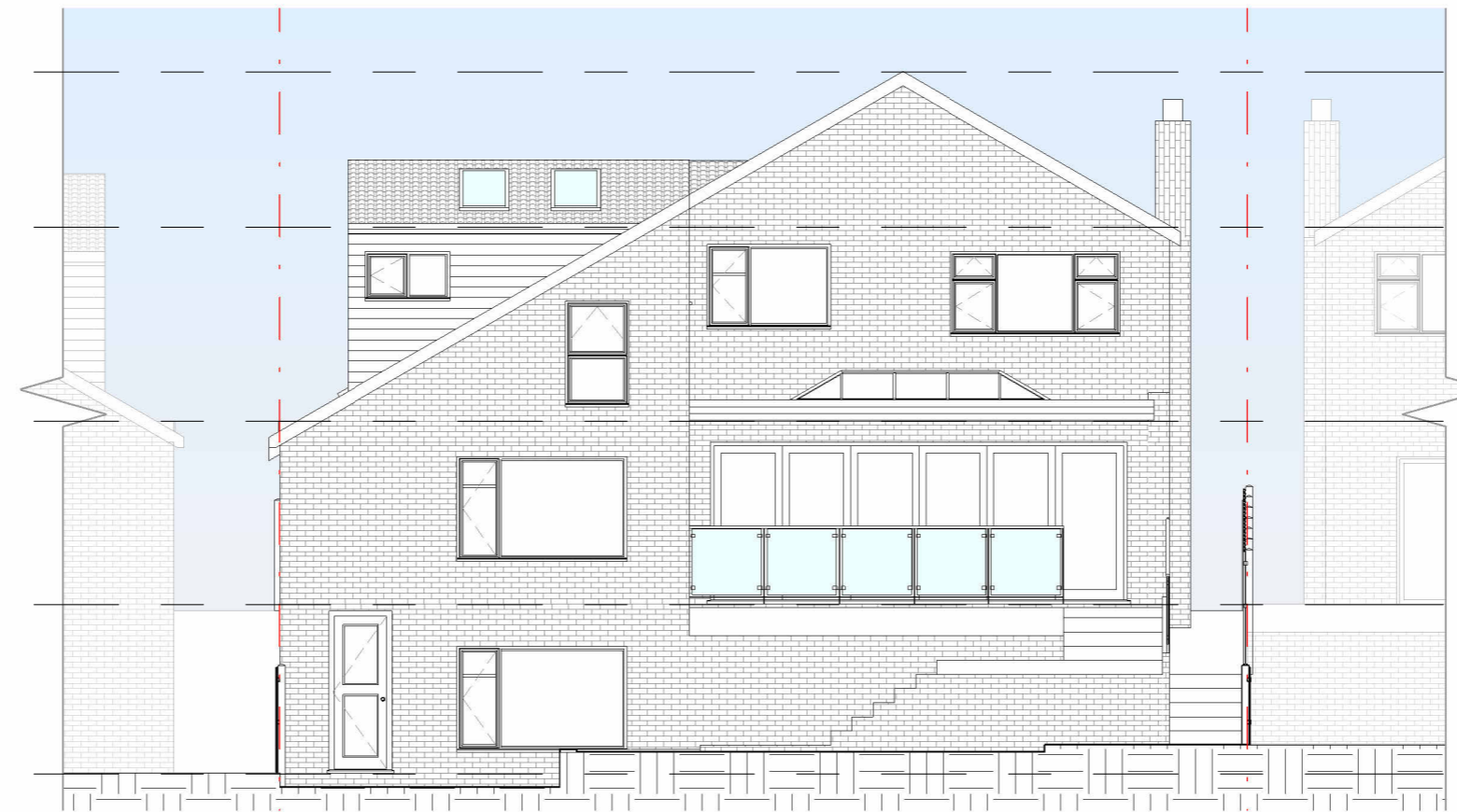
2 Existing Rear Elevation 1 : 100
